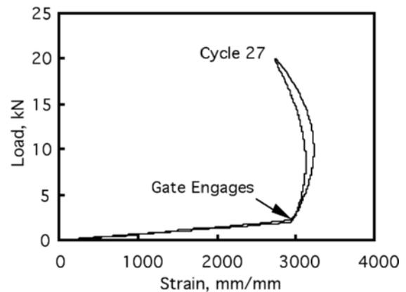
**Figure 6** Load/spine strain plot for one cycle of a 20 kN loading test
