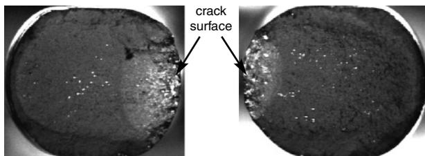
**Figure 8** Fracture surface photographs for (a) an 8 kN loading test, and (b) a 14 kN loading test. The karabiner cross-section is 1 cm × 0.8 cm. The crack initiates from the inside of the karabiner. The crack surface is the light oval patch
