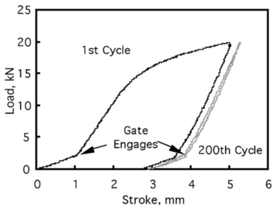
**Figure 4** Load/stroke plot for two cycles of a 20 kN loading test
