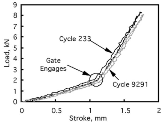
**Figure 5** Load/stroke plot for two cycles of an 8 kN loading test
