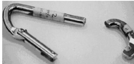
**Figure 10** Fracture location typical for all test cases
