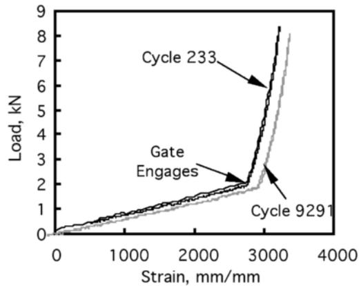
**Figure 7** Load/spine strain plot for two cycles of a 8 kN loading test
