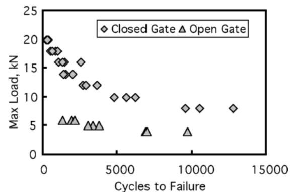
**Figure 3** Load versus cycles to failure results for closed-gate and open-gate testing
