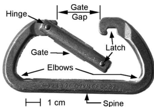
Figure 1 Karabiner used in this study with parts labelled
