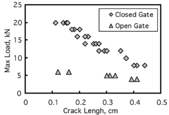
**Figure 9** Crack length measured from the fracture surface for each loading condition
