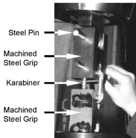
Figure 2 Photograph of test fixture. The fixture meets ASTM specification F 1774
