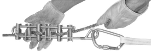
**Pulled-Back** After threading through the bars the rope is immediately pulled back toward the load as much as 180°
